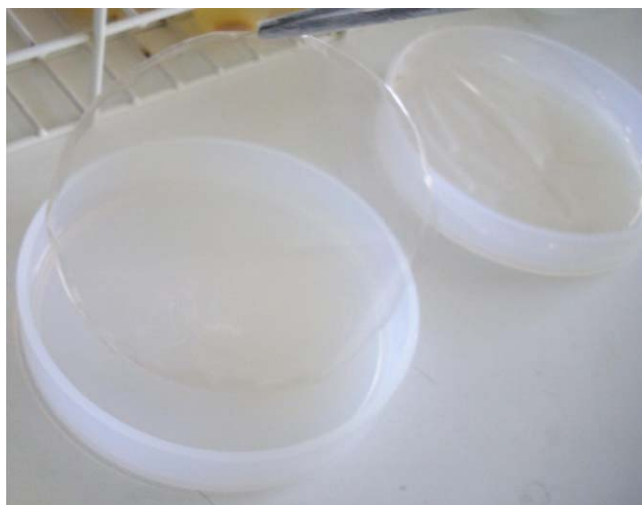
Figure 2. Film prepared with the exopolysaccharide GalactoPol by solvent casting. [Color figure can be viewed in the online issue, which is available at wileyonlinelibrary.com .]
