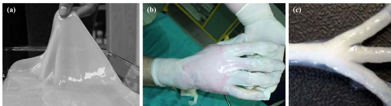
Figure 3. Bacterial cellulose pellicle produced by Acetobacter xylinum (a) and its use for the treatment of burns (b) (Reproduced from Ref. 92, with permission from Elsevier). Tubular cellulose grown on branched silicone tubing (c) (Reproduced from Ref. 93, with permission from Wiley). [Color figure can be viewed in the online issue, which is available at wileyonlinelibrary.com .]
